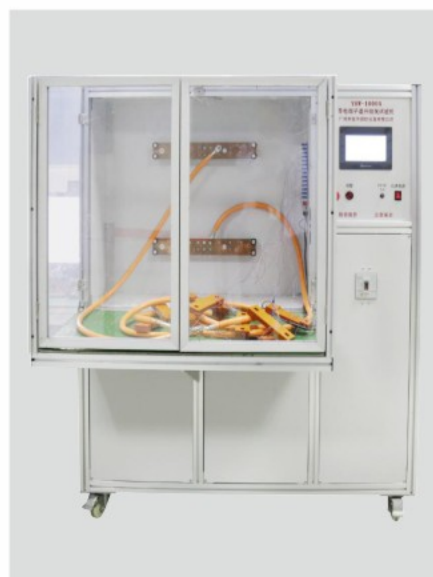
温升测试台 Temperature rise test bench
