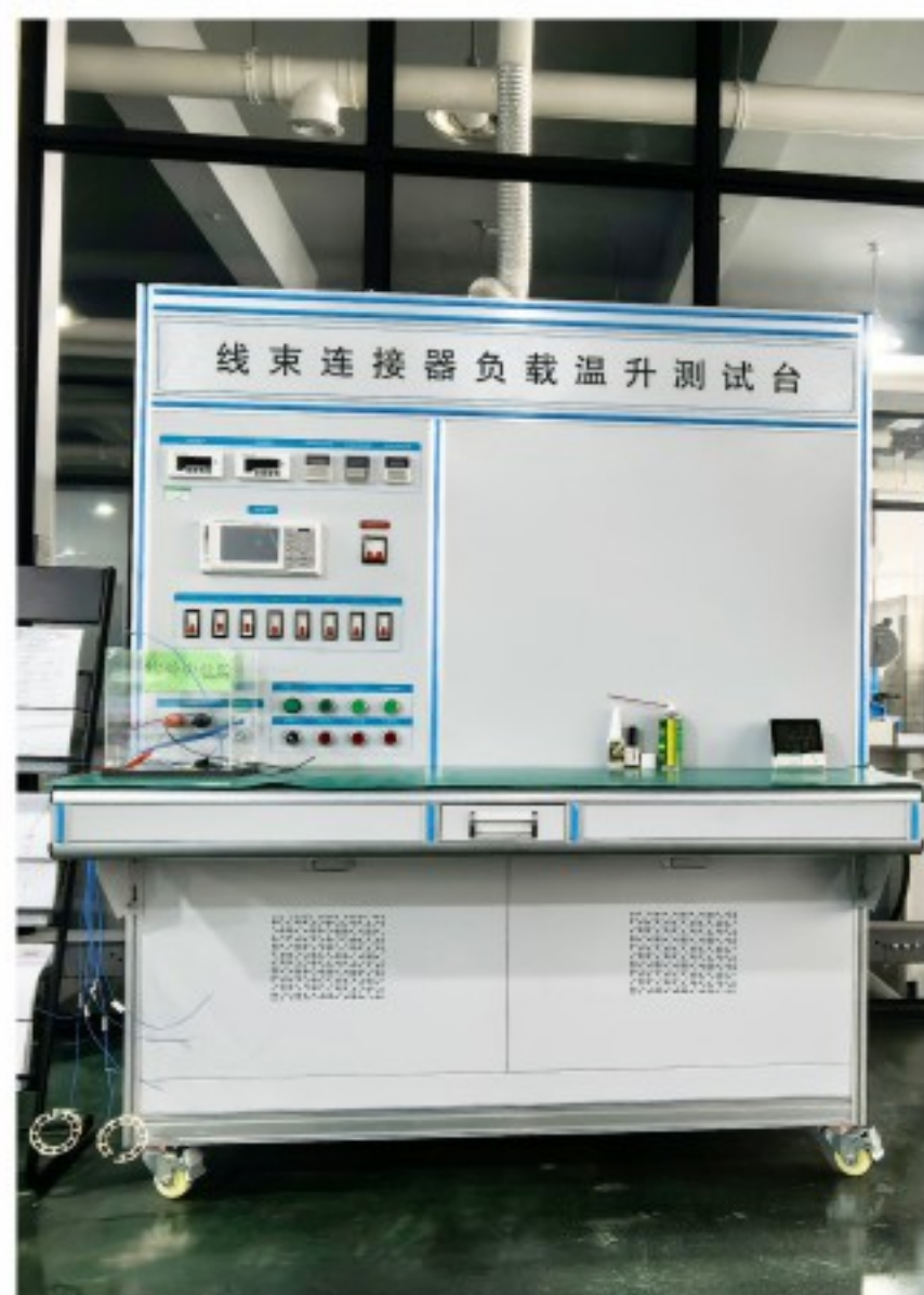
温升测试台 Temperature rise test bench
